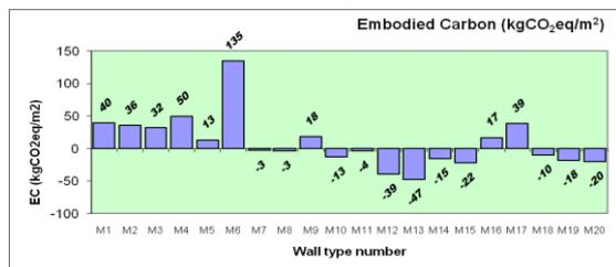
Fig 3 Embodied carbon per wall type
